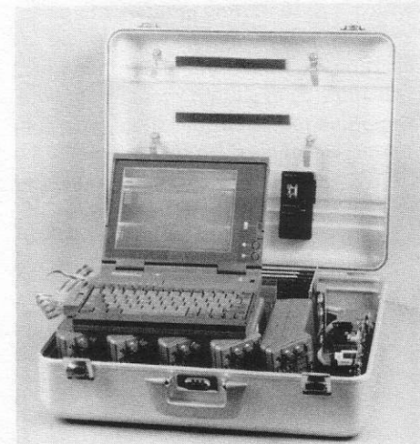
Portable configuration of the CELLTAP® cellular radio monitoring system.
