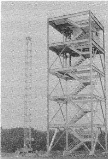
The new antenna range features a movable transmitting tower (left) and a receiving tower (right).
