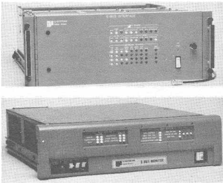
A standard E-BUS Interface (top left) combined with DEC'S LSI 11/23 (bottom left) provide system-wide analysis and maintenance.
