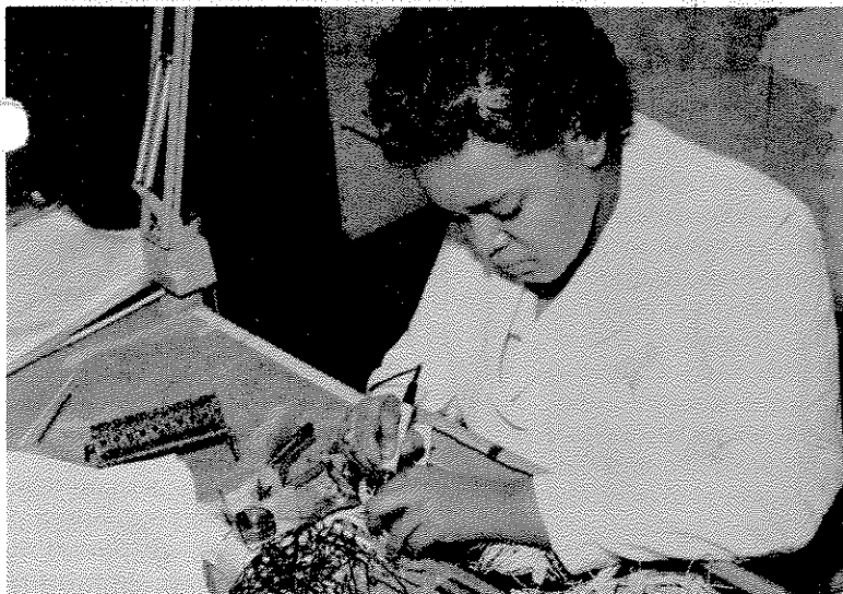
THIS ONE GOES HERE, AND . . . Following a number chart, Light Assembler Grace Ford solders the wires of an electronic system into place.
