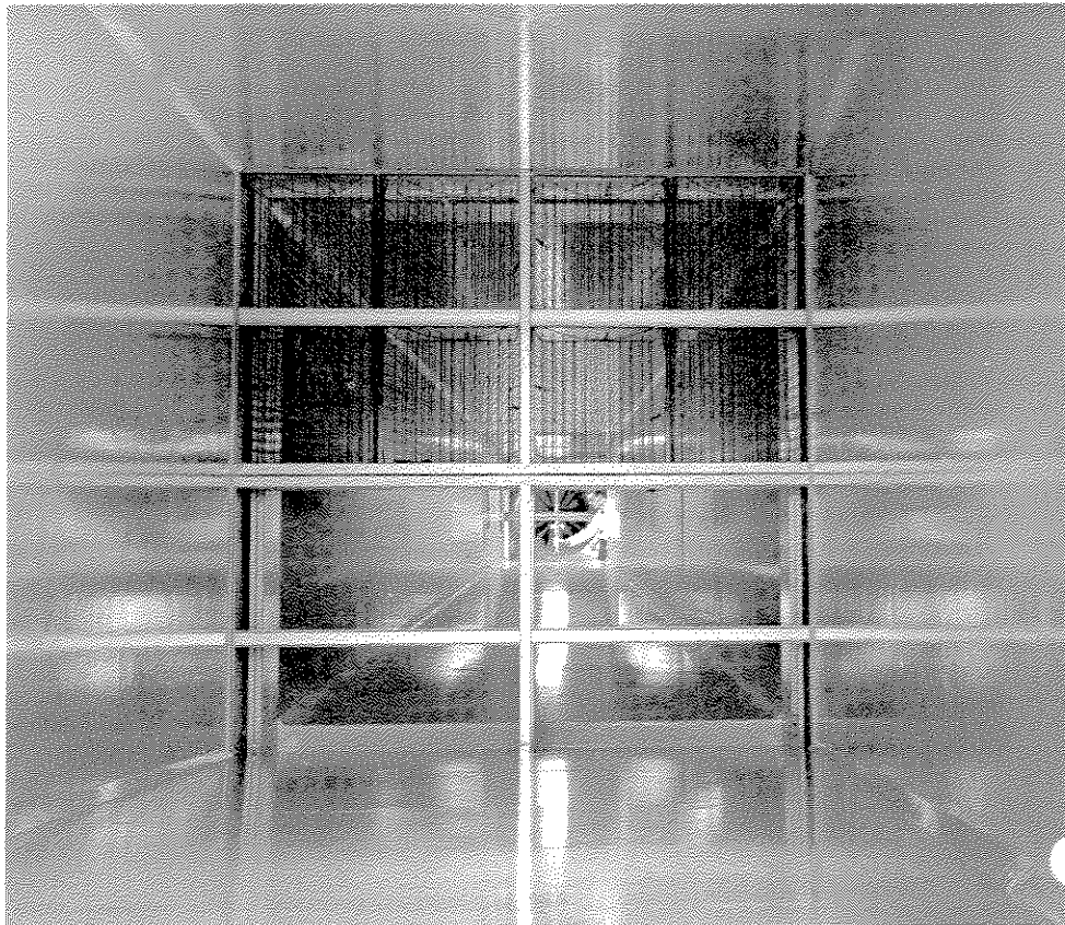
PERSPECTIVE. Reflections add interest to the geometric pattern made by the walls and grids of this aerosol test facility, now nearing completion at the Shirley Research plant. Ron McKenzie is shown placing an anemometer in what is called a working section. A preliminary study of air-flow characteristics at various wind speeds is under way.
