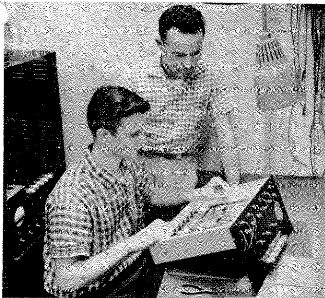
CHECK POINT . . . Electrical Technician James Orris checks a test jig circuit solder joint under the watchful eyes of Junior Engineer Richard Davis. The unit is being built by the Test Equipment group for one of the Company's major programs.
