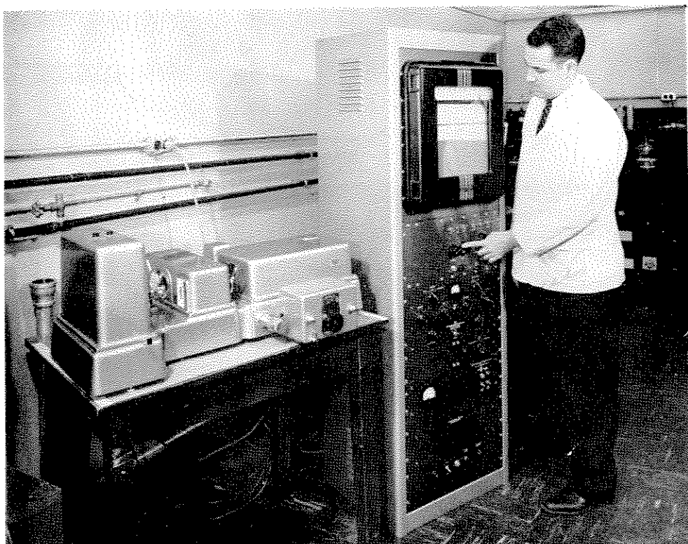
ACTUATING the Perkin Elmer Spectrophotometer is Lead Chemist S. R. Lewis, of Falls Church. The instrument rapidly identifies material through characteristic absorption patterns. Photo by Norton
