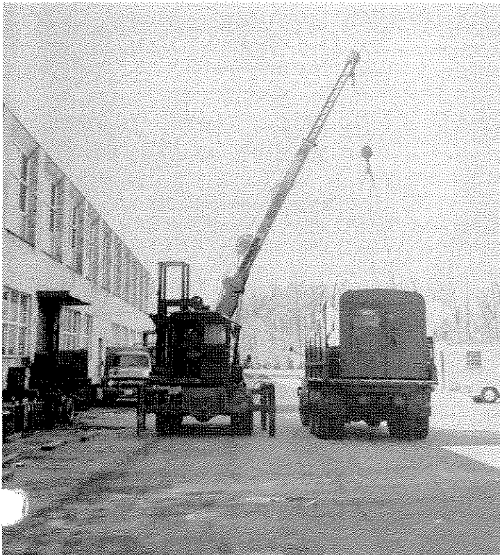
ALLEZ-OOP . . . Being lifted into position is one of two shelters containing a radically new radio-teletype system designed to combat both natural and man-made interference. The shelters, each weighing three tons, were then bolted to the bed of the truck to prevent shifting.
