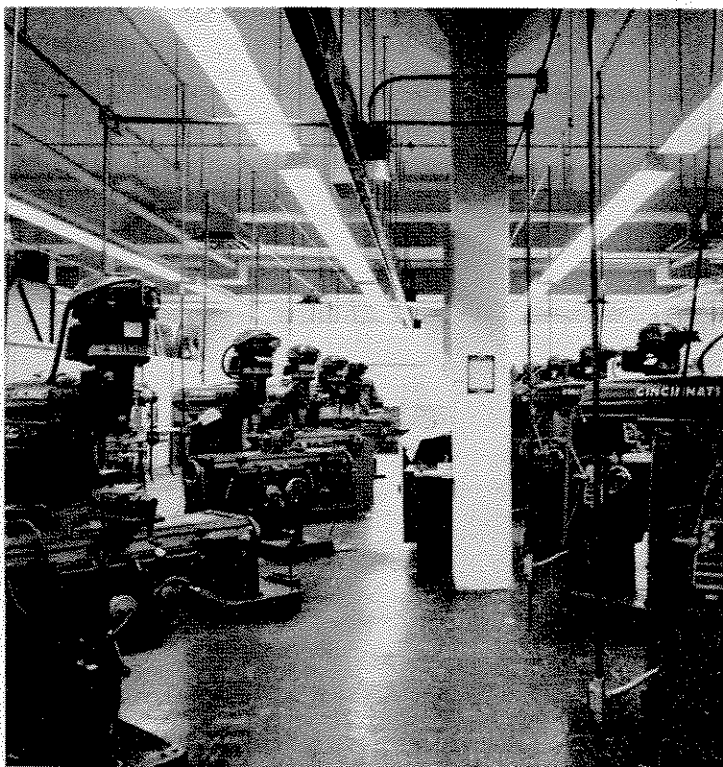
MORE MILLING MACHINES than are visible even in this wide angle photograph exploit still further the theme of flexibility and precision which governs the Company's equipment planning. These Cincinnati Millers are real quick-change artists.
