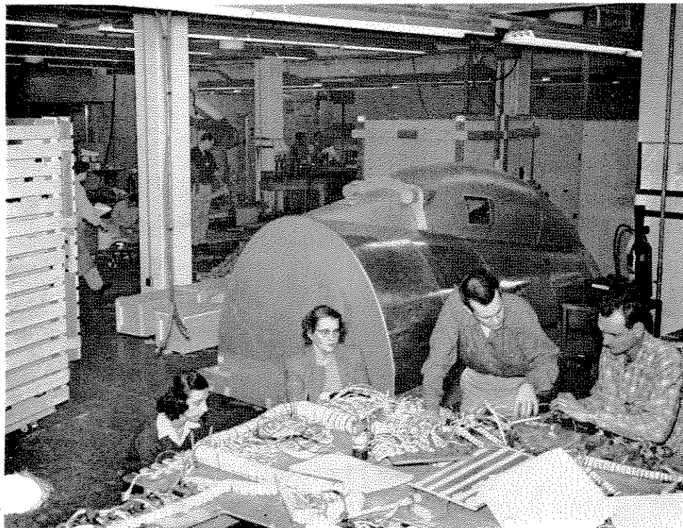
IT'S ALL THE SAME simulator job, though slightly different stages are pictured here. While the first RF-101A Simulator stands ready to go in the background, one of the cable harnesses for another gets a good going-over from (left to right) Mary Williams, Dorothy Blackburn, Frank Mahoney, and Velmer Sirman.
